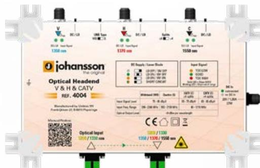
The new **Optical Compact Headend** converts Wideband/CATV signals to multiple optical wavelengths. Thanks to built-in Automatic Gain Control (AGC) and Automatic Slope Control (ASC), the output signal is of optimal quality for your optical distribution system. The 4004 can be used in combination with the 4002. Combined, they both serve as a headend for the fiber system with 5 wavelengths.
