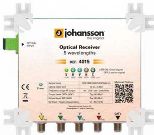
The **Optical Quintuple Receiver** is developed for the transmission of broadband signals in medium and large Fiber Optic systems. Ref.4015 converts 1310 + 1330 + 1350 + 1370 + 1550 nm to 2 x V/H and CATV signal.
